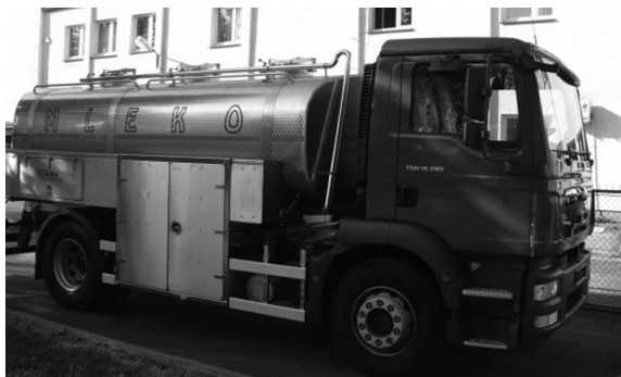
Figure 6. Tank with chest section on MAN chassis Rysunek 6. Source: [WSK „PZL – KROSNO” S.A.]
