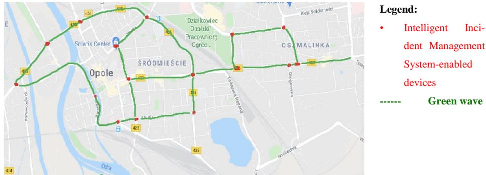
Figure 8. Graphical layout plan for traffic signal control system.
