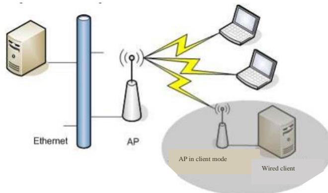
Figure 9. A Network with infrastructure (AP in customer mode, wired client)
