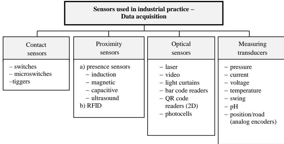
Figure 2. The division of sensors used in industrial practice for collecting data
