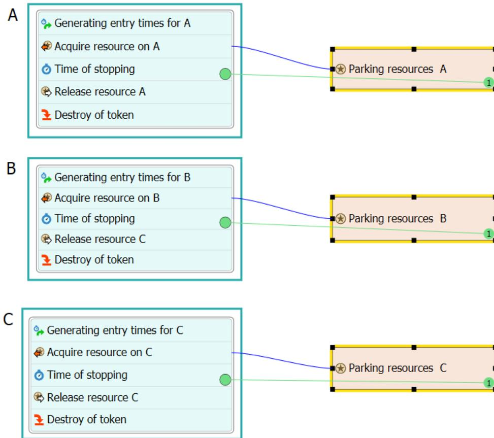
Figure 4. Block diagram of the computer model for the implementation of events in car parks A, B, C
