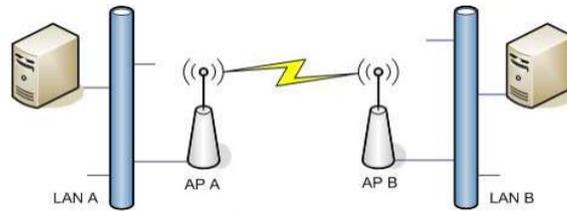
Figure 10. Bridge point-to-point
