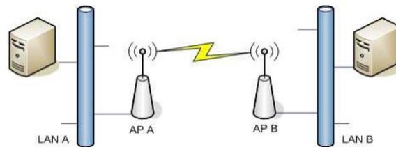
Figure 10. Bridge point-to-point
