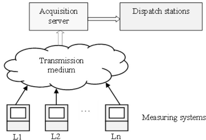
Figure 1. Example of a remote reading system
