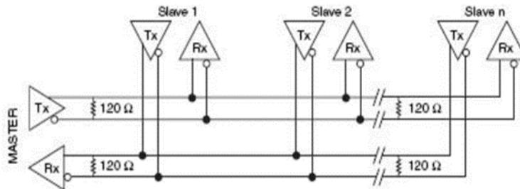
Figure 5. A bus in the Master Slave mode full-duplex
