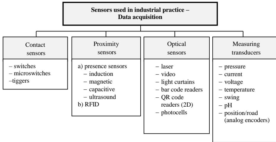
Figure 2. The division of sensors used in industrial practice for collecting data
