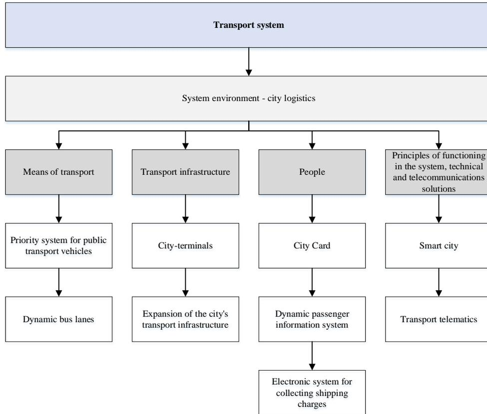
Figure 5. System environment diagram for Intelligent Transport Systems
