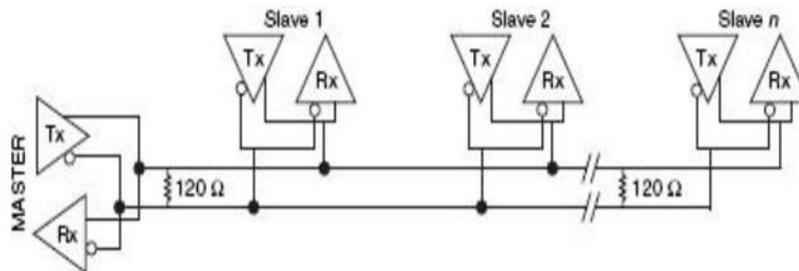
Figure 6. A bus in the Master Slave mode half-duplex
